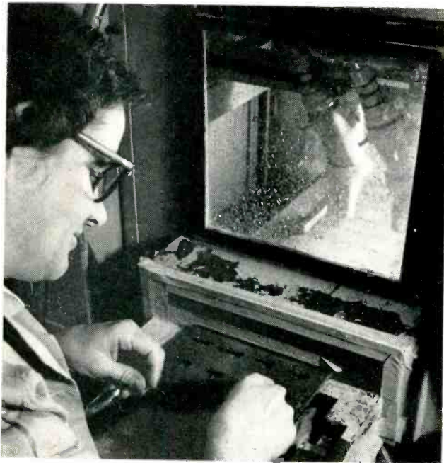
Behind strong glass, four blasts of cracked shells knock enamel off fine wire on one side of flat coil in each recess of conveyor belt
