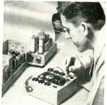
Checker finds grid-emission defects that do not show up under conventional tube tests
