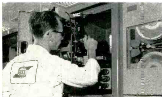
Speed change on the Ampex FR-100 is accomplished quickly and easily by a selector knob and switch.
