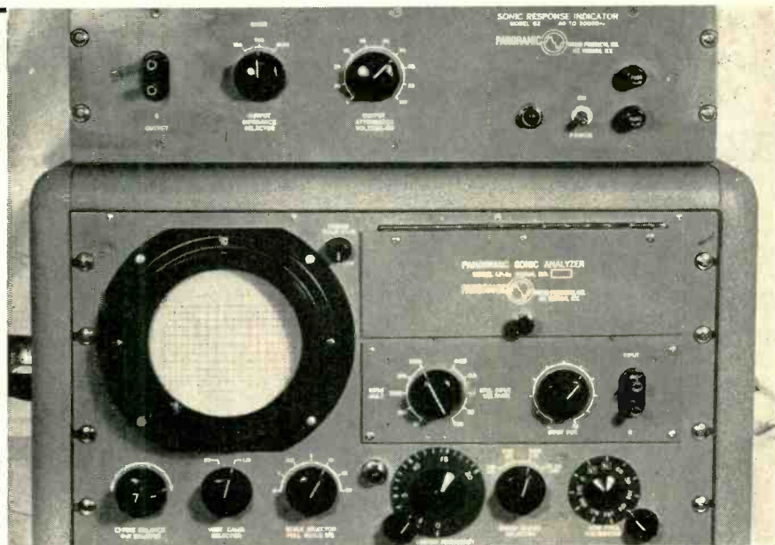
Panoramic sonic analyzer serves as selective indicator for sweep generator in the 20 to 20,000-cps range when measuring attenuation characteristics of networks
