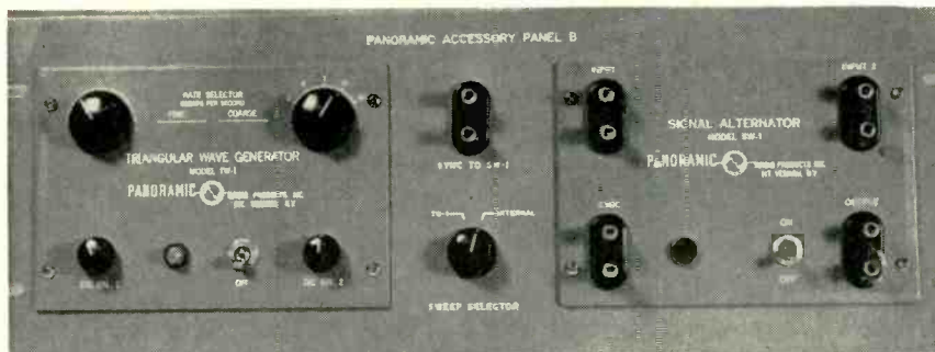
Rack-mounted triangular-wave generator and signal alternator provide variable scan and ability to compare signals for precise measurements
