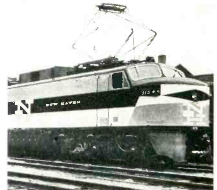
New locomotive using ignitron rectifiers to supply d-c to traction motors
