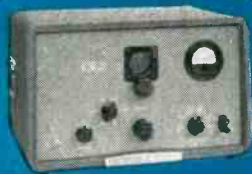
550A — highly stable, wide band; 10 cps to 10 MC. For audio, supersonic, video, rf. measurements. Output 15 mw/3 volts. Frequency response flat \pm 1 db. $490.00.
