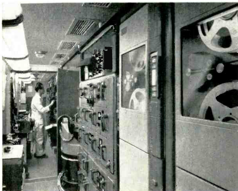
Bell Aircraft Corporation's magnetic-recorder installation aboard the SS Mariposa for study of ship motion.
