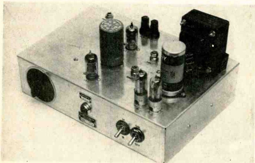
Amplifier drives Esterline-Angus recorder from output of radioactive corona point on top of flagpole. Typical fair weather value of corona current is 0.03 \mu\text{a}
