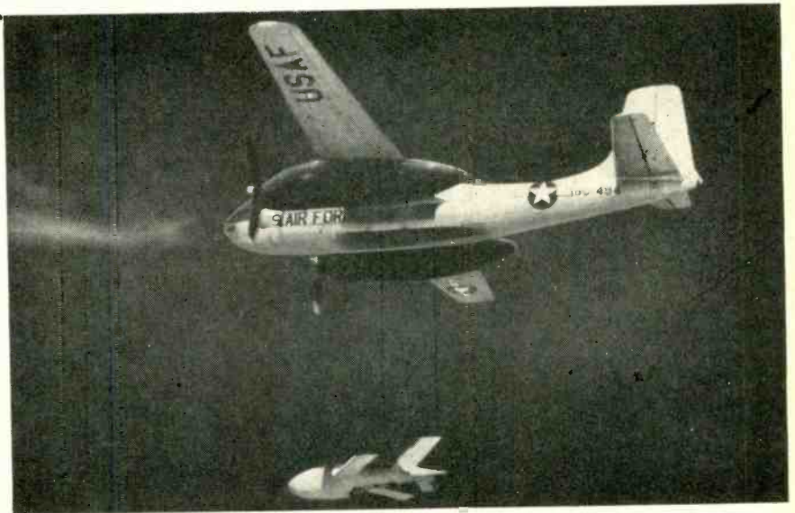
Turbojet drone dropped from plane is ground-controlled target for missile tests
