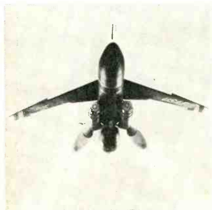
Business-end of Air Force's Snark intercontinental missile which uses an inertial guidance system. In the 5,000-mile-range category, the missile has overall length of 69 feet
