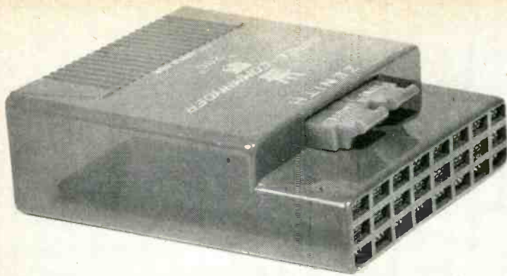
Complete two-channel transmitter, showing grille for ultrasonic output, and mounting details of aluminum rod, steel hammer and bent plastic-covered wire used as damper to terminate vibration of rod when pushbutton is released
